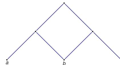
The pantograph is a well-known linkage on the Euclidean plane. If the vertex  $a$  is pinned down to the origin of the plane, then the vertex  $b$  is the image of the vertex  $c$  by a homothety of ratio  $1/2$ .
