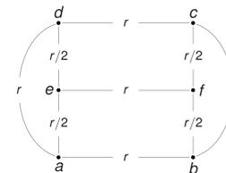
The rigidified square linkage, with one fixed vertex  $a$ , has a configuration space diffeomorphic to  $S^1 \times S^1$  on the Euclidean plane and the Minkowski plane, but it is diffeomorphic to  $S^1$  on the sphere and the hyperbolic plane.
