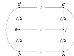
The rigidified square linkage, with one fixed vertex  $a$ , has a configuration space diffeomorphic to  $S^1 \times S^1$  on the Euclidean plane and the Minkowski plane, but it is diffeomorphic to  $S^1$  on the sphere and the hyperbolic plane.
