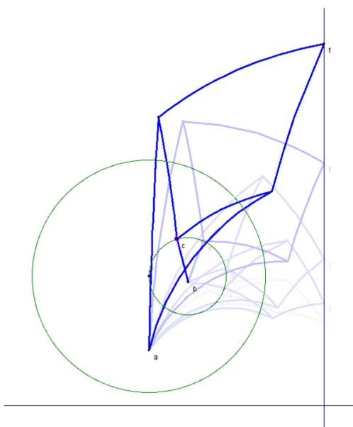
Figure 3: A straight-line linkage on the Poincaré half-plane model of the hyperbolic plane. It transforms a circle into a straight line: it is able to draw any geodesic or horocycle. In fact,  $f$  is the image of  $c$  by an inversion with respect to a circle.
