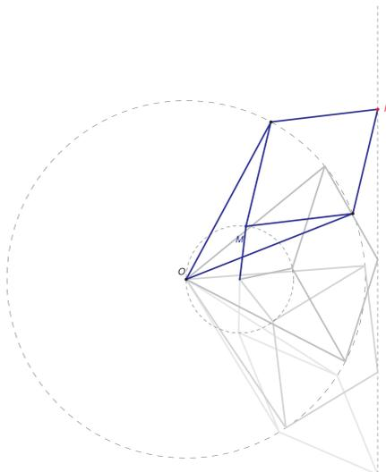
Figure 1: A straight-line linkage on the Euclidean plane. It transforms a circle into a straight line.  $M$  is the image of  $M'$  by an inversion with respect to a circle.
