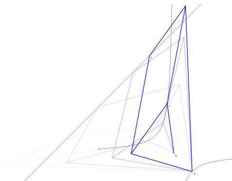
Figure 2: The Peaucellier linkage on the Minkowski plane. It transforms a hyperbola into a straight line. Three of the edges are "timelike" while four of them are "spacelike". This linkage is not able to draw "lightlike" lines.
