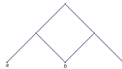
The pantograph is a well-known linkage on the Euclidean plane. If the vertex  $a$  is pinned down to the origin of the plane, then the vertex  $b$  is the image of the vertex  $c$  by a homothety of ratio  $1/2$ .
